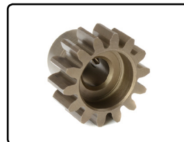
C-72714 Pignon M1.0 - Acier Dur - 14 Dents - Axe Dia. 5mm
